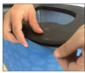
8. Pull graphic taut and angel and tuck gasket into channel in edge of foot. Insert graphic gasket all the way around.
