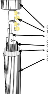
Case lid Pack bulbs in boxes Two light bars, slide and lock connector bar flush with end. Cardboard tube
